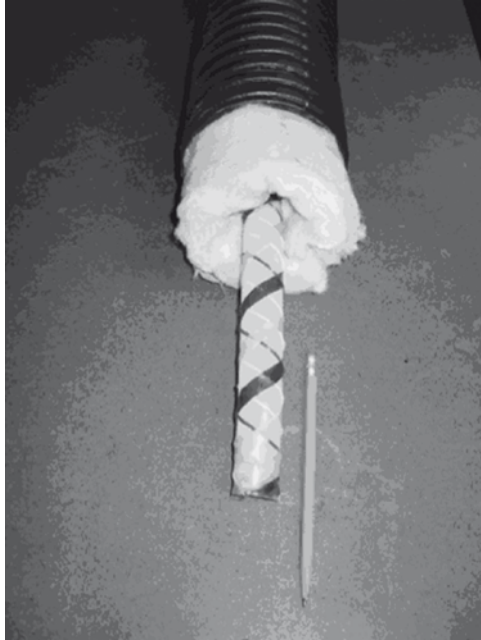
Fig. 5.15 Photo of the optical fiber infrasound sensor. The sensor is a 2.54 cm diameter silicone tube wrapped with two optical fibers. A laser shines through the fibers. The sensor measures pressure induced diameter changes of the silicone tube with laser interferometry
