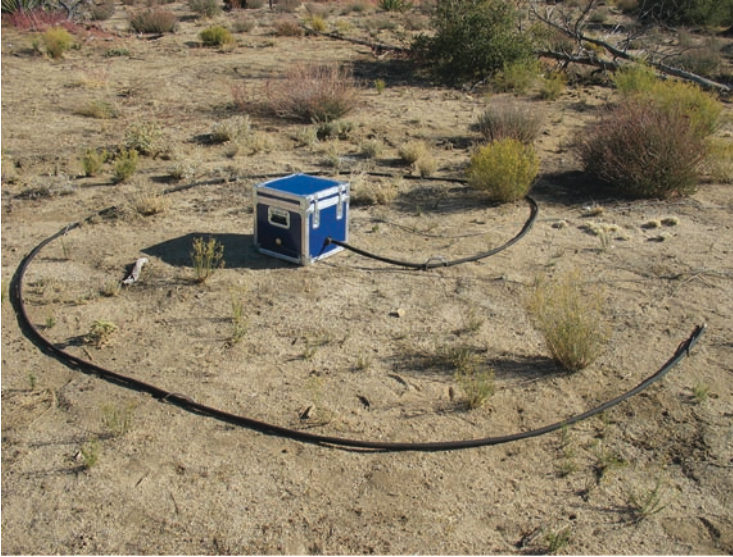
Fig. 5.14 Photo of a spiraling-outward microporous hose connected to a microbarometer at Piñon Flat Observatory
