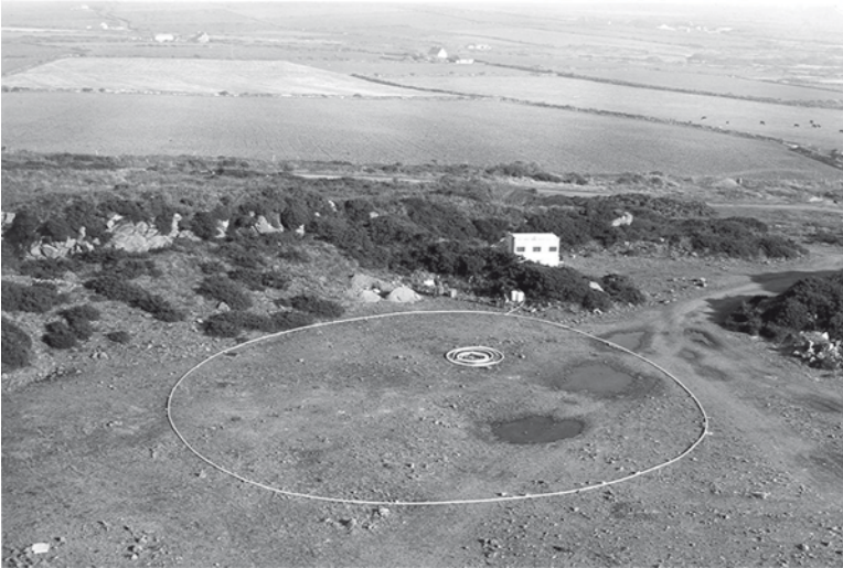
Fig. 1.15 Thirty-hole ring array at the sonic boom effects recording site in the UK, from Grover (1971)
